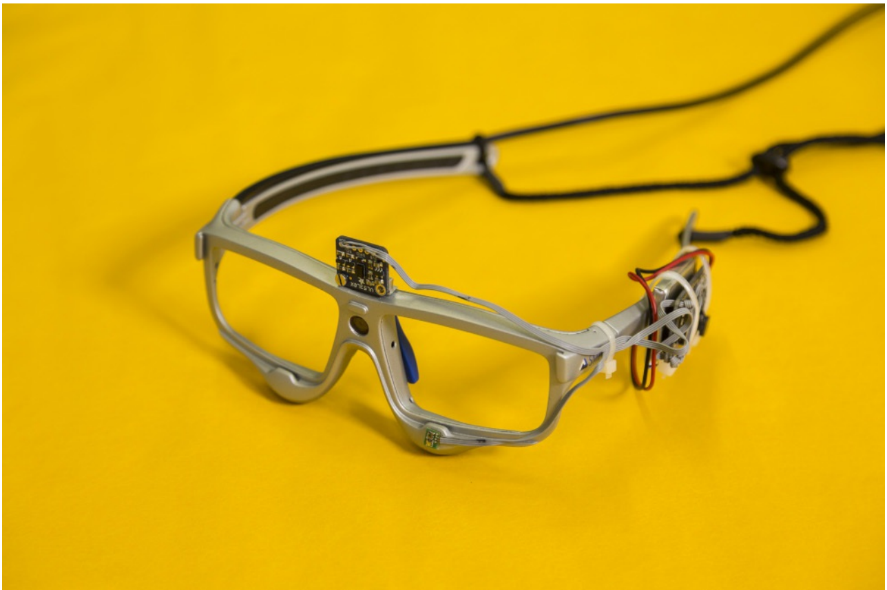
Smart glasses developed by Leung and Schmied, which measure both light effects and eye movements.
