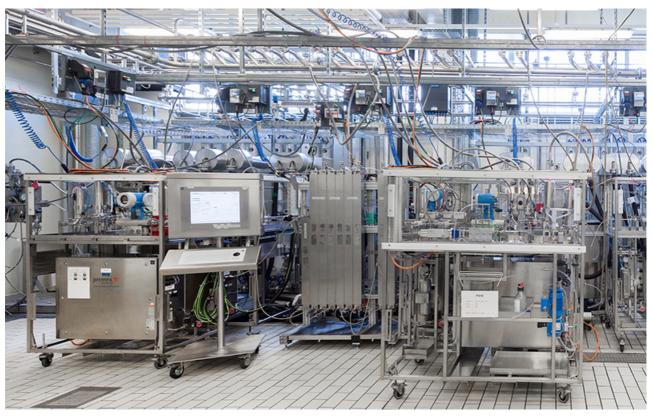
With continuous manufacturing, chemicals flow through multiple vertical chemical reactors that perform sequential reactions. Computer software controls the reactions and assesses quality. Image by Tanja Devald/Novartis.
