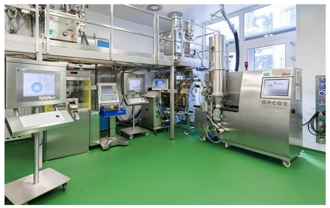
Once the chemical reactions are complete, pill production begins. The system dries and granulates the active substance and compresses it into tablets. Image by Tanja Devald/Novartis.  $2\!/\!3$
